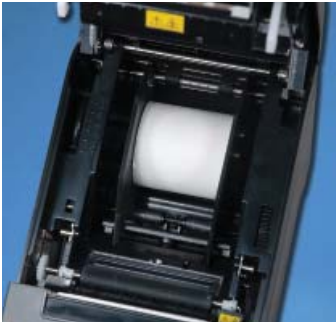
Drop and Print Paper Loading with an Adjustable Paper Width Selector
